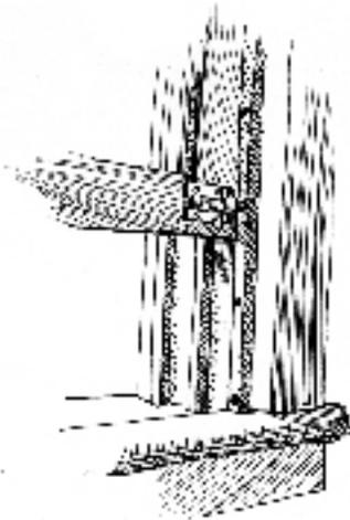
One option is to attach slide bolt on the bottom of the sash. Then mark three or four spots on the inside stop by tapping the bolt with a hammer. Drill holes slightly larger than the bolt at the marks .
