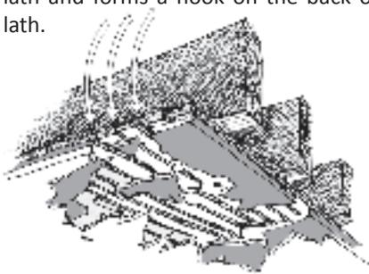
**3** Where the plaster keys are broken and plaster is pulling away from the lath, tighten loose plaster back to the lath with plaster washers. Where possible squeeze construction mastic through holes between plaster base-coat and lath. To hold assembly while drying wedge a 2x4 between the floor and a square of plywood held against the ceiling.
