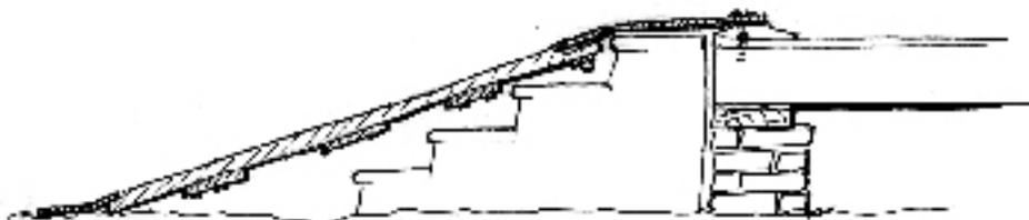
Screw top of ramp to threshold, floor, or top of steps.
