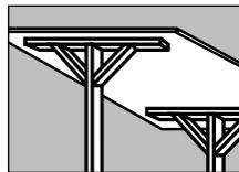
One piece of the 1 x 4 should be used for the top of the "T", while the second piece should be used as a brace and attached diagonally from the top piece to the stem. You'll need to make sure the T stays square.
