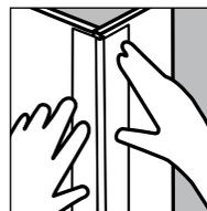
Measure bead and cut to right length; a snug fit from floor to ceiling (about 1/4" shorter than the wall height). With a 7" knife apply a generous amount of CertainTeed joint compound on either side of corner. Using even pressure, press paper / metal bead onto corner into position, ensuring it is aligned; embed it into
