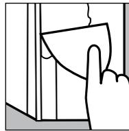
compound by running the knife at 45° angle. Let dry for 24-hours. Apply a second coat with the 7" knife, allowing knife to rest on nose of the bead. Let dry for 24-hours and apply a third coat. After another 24-hours, sand the corner to a smooth finish.
