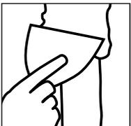
Apply a second coat using a 7" tapping knife and this coat should extend approximately 4" – 6" beyond each side of the joint.
