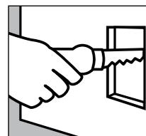
For larger openings, install the panels directly across the openings. Then use a drywall saw to cut the panels, using the framing as your guide. As you install the boards, make sure that you do not place joints at the edges of doors or windows. If you do, as the door or window is opened and closed over time, the joint will crack.
