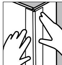
To prepare the corner for finishing, install a corner bead. Measure the length needed, then cut the bead with tin snips, cutting through each flange towards the nose, then bending the bead to break. After
