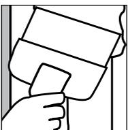
Apply a third coat using a 12" tapping knife and this coat should be a thin coat and should extend approximately 7-12" beyond each side of the joint. The further
