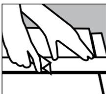
CertainTeed drywall is very easy to work with and cutting is quite simple. To make a cut, score the paper on the face side with a utility knife along the edge of your T-square. Apply firm, but even, pressure to snap the board along the score. Then fold the board along the score and cut the paper along the crease with the utility knife. Lastly, smooth the rough edges with a sanding block or drywall rasp.
