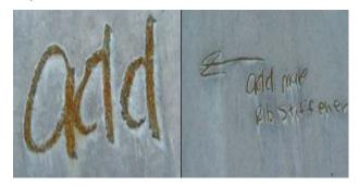
Figure 10-45 Corrosion Caused by Graphite Pencil
