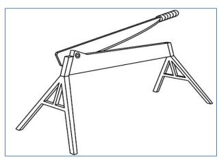
Figure 12-4 Shear, or Trimmer, For On-Site Use
