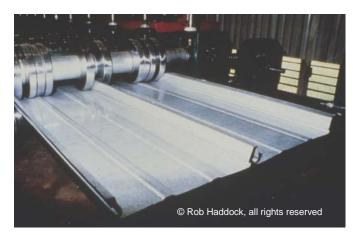
Figure 2-8 Roll Forming Equipment
