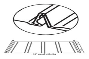
Figure 4-12 Example of Interlocking Side Seam
