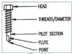
Figure 14-1 Key Areas of a Typical Fastener
