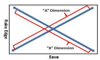
When the corner to corner dimensions of a rectangle are equal; the sides are square to each other.
