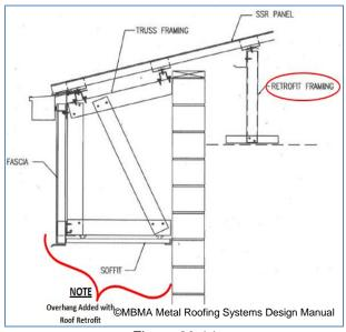
Figure 20-14 Sidewall Overhang Added During Retrofit
