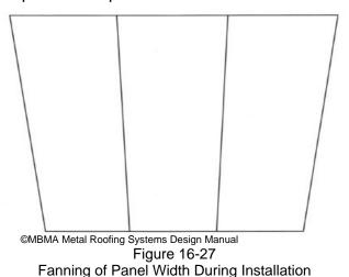
There is no assurance, other than the care of the installer, that a panel will cover its intended dimension. Most panels tend to gain dimension, not lose it.
