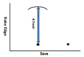
Step 4 - From the first nail, measure exactly 4 feet straight up the slope of the roof and draw a small arc.
