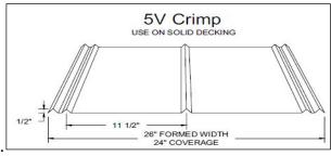
Figure 5-1a Formed vs. Coverage Width
