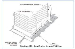
Figure 10-66 Apron Flashing Around a Chimney
