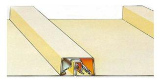
Figure 4-8 Modern Batten Seam with Snap-on Cover Note – No Wooden Batten
