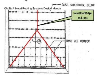
Figure 20-3 New Ridgeline with Retrofit
