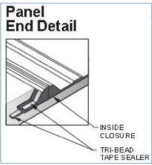
Figure 13-27 Closure Sealing of Panel Closure
