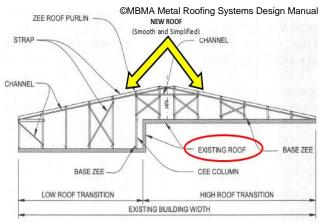
Figure 20-2 Simplified Roof-Line from Retrofit
