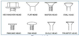
Figure 14-3 Fastener Heads
