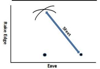
Step 5 - Measure from the second nail exactly 5 feet and draw an arc that intersects the first arc.
