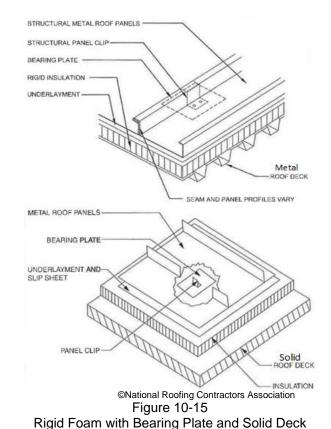
The potential for condensation to occur between the metal roof panel and the rigid insulation should be addressed during the installation. An underlayment should be installed on top of the rigid roof insulation in a manner similar to that used on a solid deck and illustrated in Figure 10-16.
