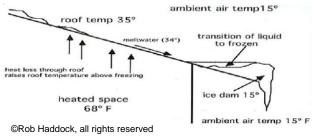
Figure 10-23 Ice Dam Formation on a Roof
