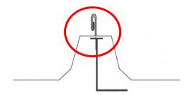
Figure 7-19 After Mechanical Seaming
