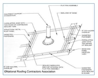
Figure 10-76 Flashing Sealant Locations
