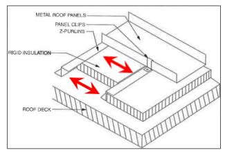
Figure 6-10 Rigid Insulation Using Z Purlins
