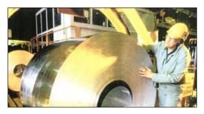
Figure 5-3 Large Coils of Sheet Metal Allow Larger Roof Panels to be Produced
