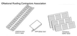
Figure 8-5 Soffit and Drip Edge Vents
