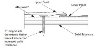
Figure 5-20 Lap Joint with Fasteners For Unitized Panels
