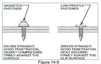
Properly Installed Fasteners Are Straight and Tight
