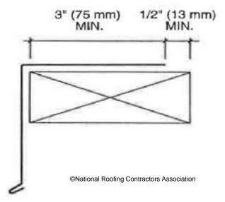
Figure 10-55 Nailer Details for Drip Edge Material
