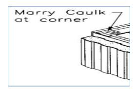
Figure 13-24 Marrying Sealants at Eave Prevents Leakage
