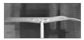
Figure 10-39 Over-Driven Fastener
