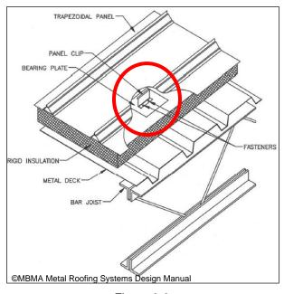
Figure 6-9 Rigid Insulation Using Bearing Plates
