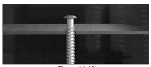
Figure 14-10 Under-Driven Fastener
