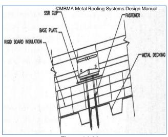
Figure 14-22 Clips Installed Over Rigid Foam May Require Different Fasteners and Base Plates
