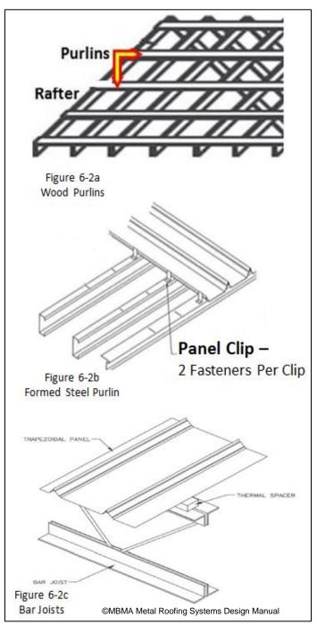
Figure 6-2 Common Open Framing Styles
