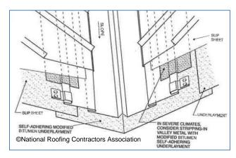
Figure 10-70 Stripping of Clip-Installed Valley Trim
