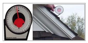
Figure 10-85 Slope Measurement Tool
