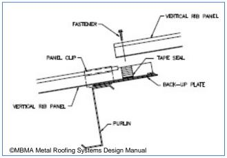
Figure 10-72 Endlap Sealant Locations
