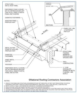
Figure 10-62 "L"-Type Downslope with Gutter & Straps
