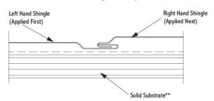
Figure 5-19 Side Lap Joint for Unitized Panels
