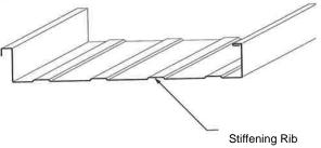
Figure 4-16 Vertical Rib Profile
