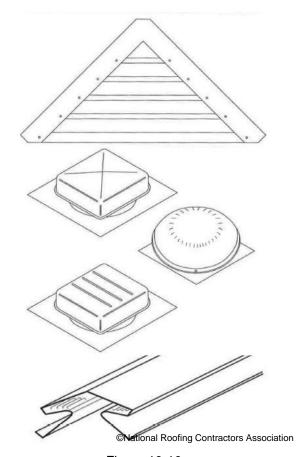
Figure 10-10 Examples of Common Ridge and Gable Vent Styles
