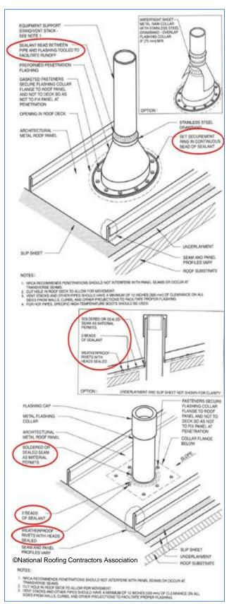
Figure 13-20 Roof Penetration Sealing Examples
