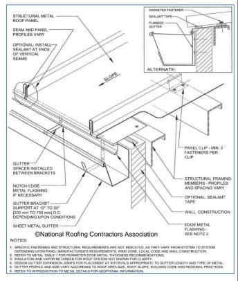
Figure 10-65 "T"-Type Downslope with Gutter and Brackets
