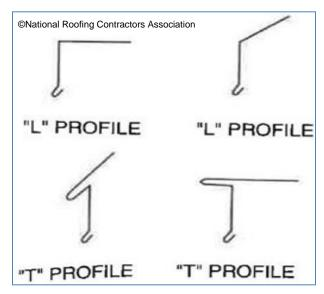
Figure 10-50 L and T style Drip Edge Profiles
