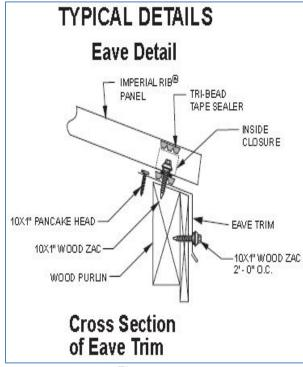
Figure 13-28 Eave Sealing Details
