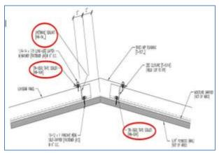
Figure 13-25 Ridge Sealant Example
