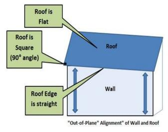
Figure 16-8 Incorrect Alignment of Roof and Wall
