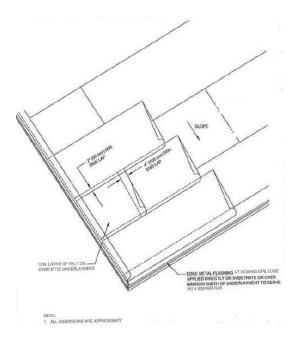
Figure 10-16 Underlayment over Rigid Insulation
