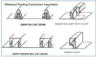
Figure 15-10 Snap Seam Profile Examples
