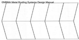
Figure 16-18 Dog-Legging of Multi-Tiered Roof Panels
