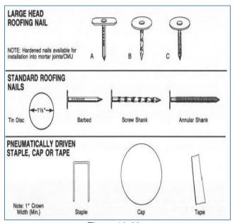
Figure 10-29 Underlayment Fasteners
