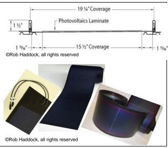
Figure 8-33 BIPV Laminated Thin Film
