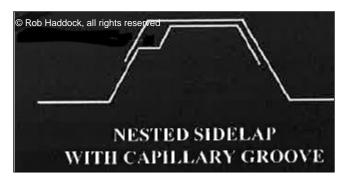
Figure 15-4 Addition of a Capillary Groove to a Nested Seam
