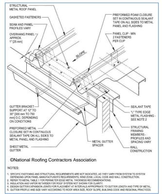
Figure 10-61 "L"-Type Downslope with Gutter and Brackets
