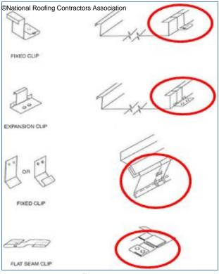
Figure 14-21 Common Clip Styles and Installation
