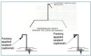
Figure 13-7 Pre-Applied Sealant
