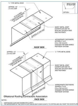
Figure 13-22 Flashing Cover Plate Sealing
