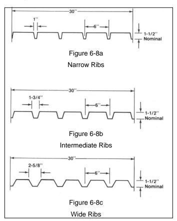
Figure 6-8 Common Rib Profiles
