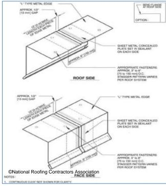
Figure 13-23 Flashing Concealed Plate Sealing
