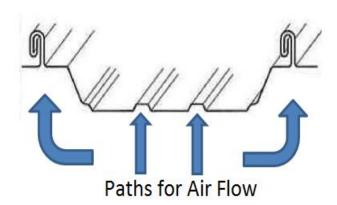
Figure 10-11 Ventilation Provided by Panel Profile
