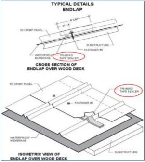
Figure 13-3 Internally Applied Sealant
