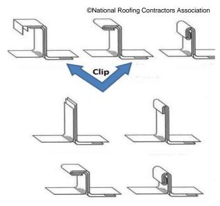
Figure 14-34 When Rolled, the Clip Becomes Part of the Seam
