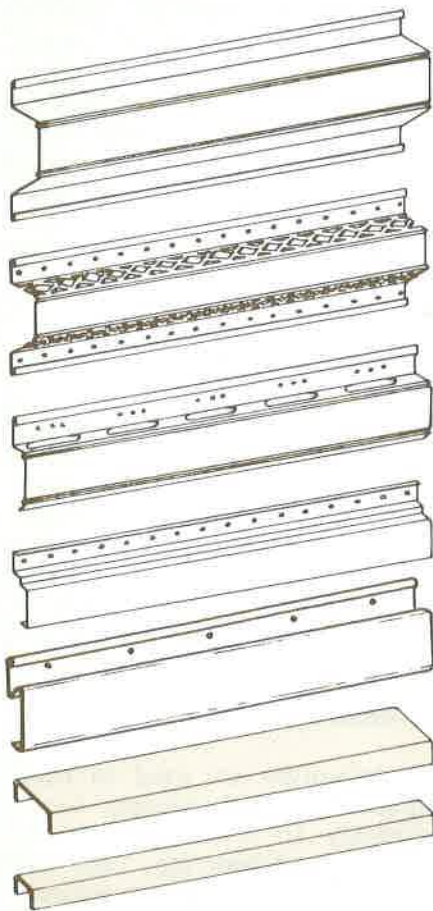
Fig. 20 Plain drywall channel (top) has a hat shaped cross section, while resilient drywall channels (center four) come in several designs. All are of galvanized steel. Cold rolled channels (bottom two) are "C" shaped and generally of 16 gauge black asphaltum painted steel.
