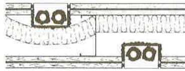
Caulking of openings through partitions
