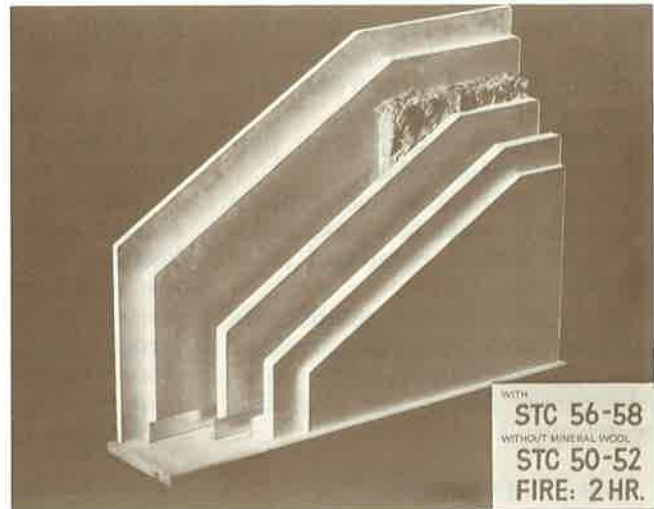
Fig. 43 Triple solid gypsum board partitions have three parallel courses and provide superior sound control when a mineral wool or glass fiber blanket is added.
