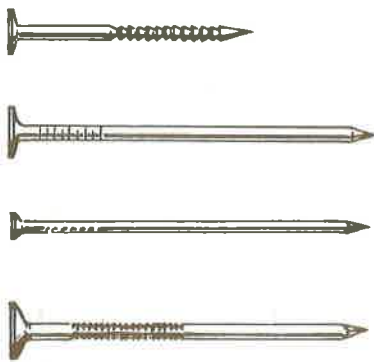
Fig. 23 Nails used in drywall construction have thin, 1/4 in. diameter heads. Small-headed nails shown are colored for use with predecorated wallboard. These are used according to instructions of the manufacturers.
